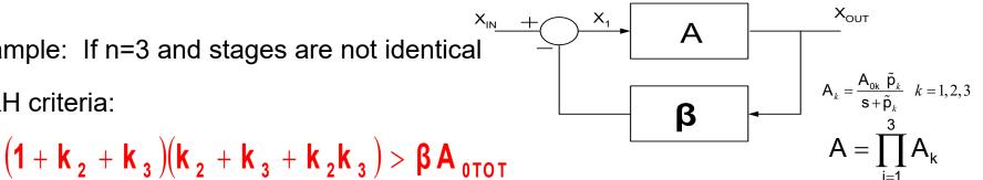
Since  $A_{0TOT}$  will, in general, be very large for the cascade of 3 stages, a very large pole ratio is required just to maintain stability and an even larger ratio needed to avoid a close to becoming unstable situation
