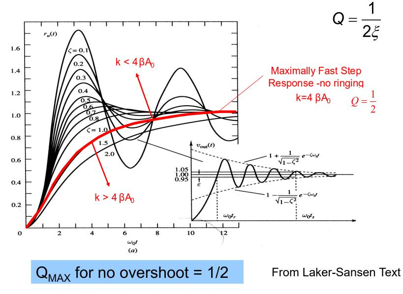
For two-stage amplifiers, must have open-loop pole spread, k, very large to avoid ringing in step response
