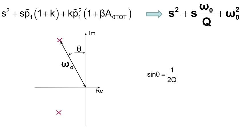
$\omega_{o}$  = magnitude of pole Q determines the angle of the pole
