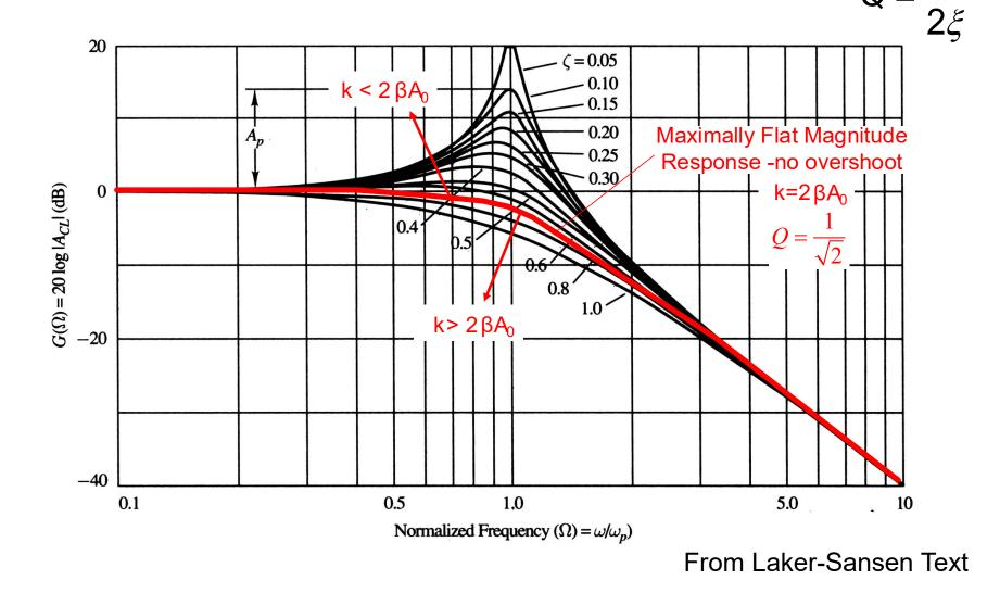
For two-stage all-pole amplifiers, must have open-loop pole spread, k, very large to avoid overshoot in closed-loop gain
