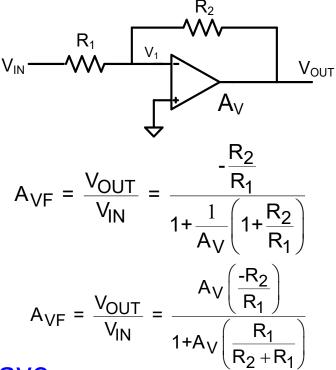
$\beta = \frac{R_1}{R_2 + R_1}$
