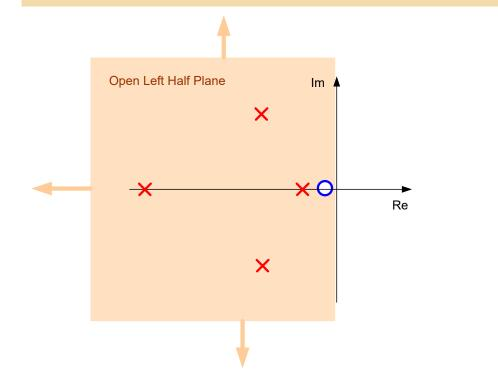
Stable with two negative real axis poles, two LHP complex conjugate poles, and two LHP CC poles Unstable with positive real axis pole
